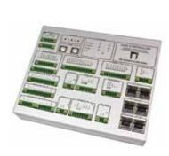
The axis controller is universally applicable and easy to maintain. All the connections are plug-in, which allows it to be easily replaced. More detailed technical data can be found on the technical data sheet.
